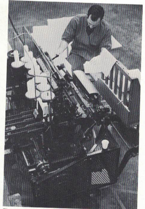
The sewing machines bind together signatures of the book.
